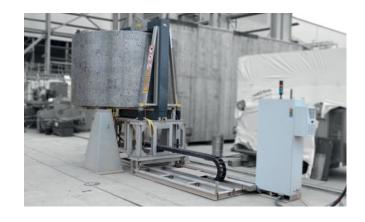
Customized heater, able to heat a 100 ton Grinding Roll to 200° C in 17 hours with low power consumption
